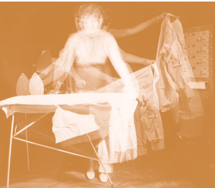
"Energy output in ironing," 1955. Photograph taken with a stroboscopic camera as part of a test at DuPont's Haskell Labs. The test revealed that a woman ironing a shirt uses twice as much peak energy as a man does painting the living room ceiling. 1972341_3891, Series XIV, Box 12, Folder 2 "Studies of Industrial Fatigue." DuPont Company Product Information photographs (Accession 1972.341), Audiovisual Collections and Digital Initiatives Department, Hagley Museum and Library, Wilmington, DE 19807.
